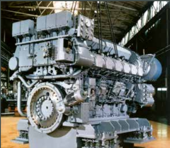
Diesel Engine with Spring Support (Spring Viscodamper® Combinations)
